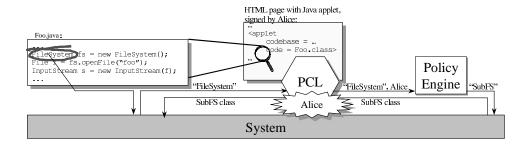
Fig. 8. Changing the name space: A PrincipalClassLoader (PCL) replaces the original class loader. The class implementation returned depends on the principal associated with the PrincipalClassLoader and the configuration in effect for that principal.
